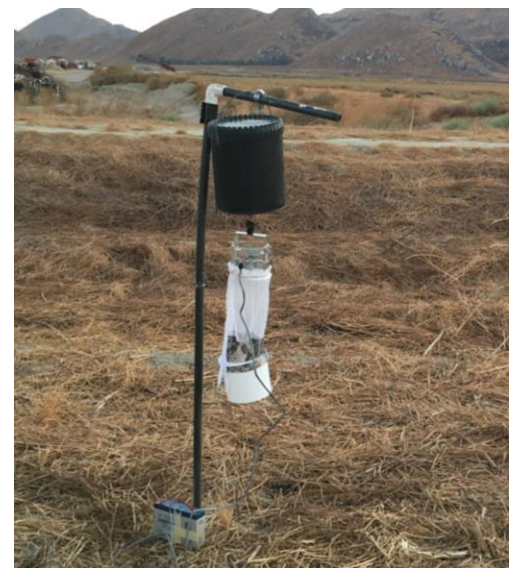
Figure 4: CDC miniature suction trap baited with dry ice (CO 2 ) to collect biting midges on a dairy farm. Photo by Xinmi Zhang, UCR, USA.
